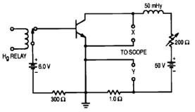
Figure 4. Sustaining Voltage Test Circuit
