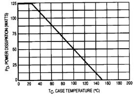
Figure 2. Power-Temperature Derating Curve
