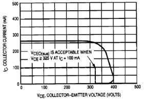
Figure 3. Sustaining Voltage Test Load Line
