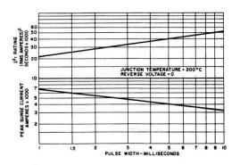
SUB-CYCLE SURGE FORWARD CURRENT AND I<sup>2</sup>t RATING VS. PULSE TIME FOLLOWING RATED LOAD CONDITIONS
