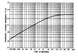
TRANSIENT THERMAL IMPEDANCE – JUNCTION-TO-CASE
